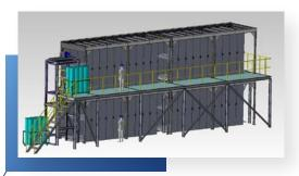
Given the space restrictions, the sleeve storage system is custom engineered to store **sleeves of different dimensions**. We suggest to use a multiple level system, the easiest to handle sleeves on the upper level. Features of the sleeve storage system include a customized steel frame that accommodates suspended sleeve racks and a holder on the ceiling that prevents the sleeves from falling off when the racks move. This system can also be expanded in the future with additional racks.
